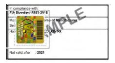
Racing seat, if original seats are changed it must be for seat system for which the FIA Homologation is valid. (FIA Technical list N° 12 and 39)
